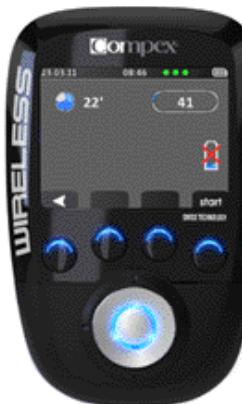
During stimulation, a module's battery may run out. If this happens, the symbol of an empty battery is displayed on the channel where the problem has been detected (in this example, channel 4).
