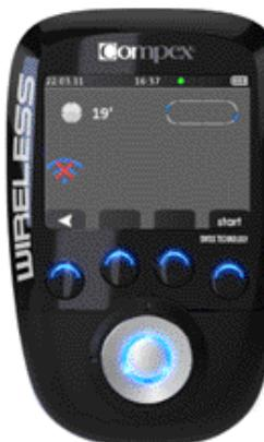
The remote control shows the out of range symbol on the channel where the problem has been detected (in this example, channel 1).
