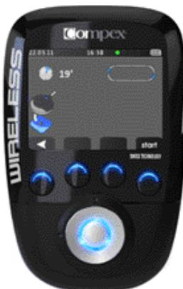
The remote control shows the symbol of an electrode and a disconnected module on the channel where the problem is detected (in this example, channel 1).
