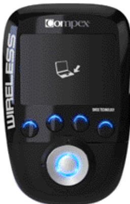
If the synchronisation process has been interrupted or if for any reason you cannot synchronise (remote disconnected, power failure, etc.), the remote control may display this screen.
